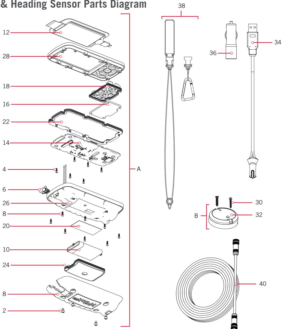
Remote & Heading Sensor Parts List
