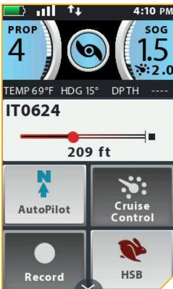
The Record iTrack Active Band appears while a recording is in progress. The boat has traveled 209 feet during the current recording.
