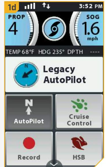
**NOTICE:** If the Prop is not turning or is flashing, be sure to press the Prop Button
