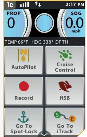
**NOTICE:** If Cruise Control is engaged, making adjustments to motor speed from the Foot Pedal or engaging High Speed Bypass will cancel Cruise Control.
