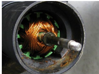
FIGURE 4 (Water damage to the lower unit)
